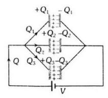
Between A and B, 3 capacitors are in series and they are in p
