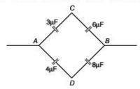
In the upper arm capacitors 3µF and 6µF are connected in series and similarly in lower arm capacitors 4µF and 8µF are connected in series . The equivalent capacitance is given by
