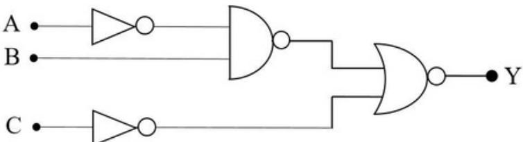
Consider the logic circuit with inputs A, B, C and output Y. How many combinations of A, B and C gives the output  $Y = 0$  ?
