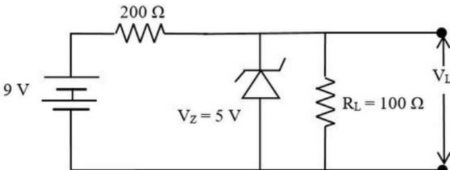
In the given circuit, find the voltage drop  $V_L$  in the load resistance  $R_L$ .
